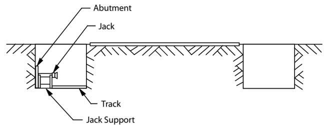
Pits are excavated on each side. The jacks will bear against the back of the left pit so a steel or wood abutment is added for reinforcement. A simple track is added to guide the concrete pipe sections. The jacks are positioned in place on supports.
