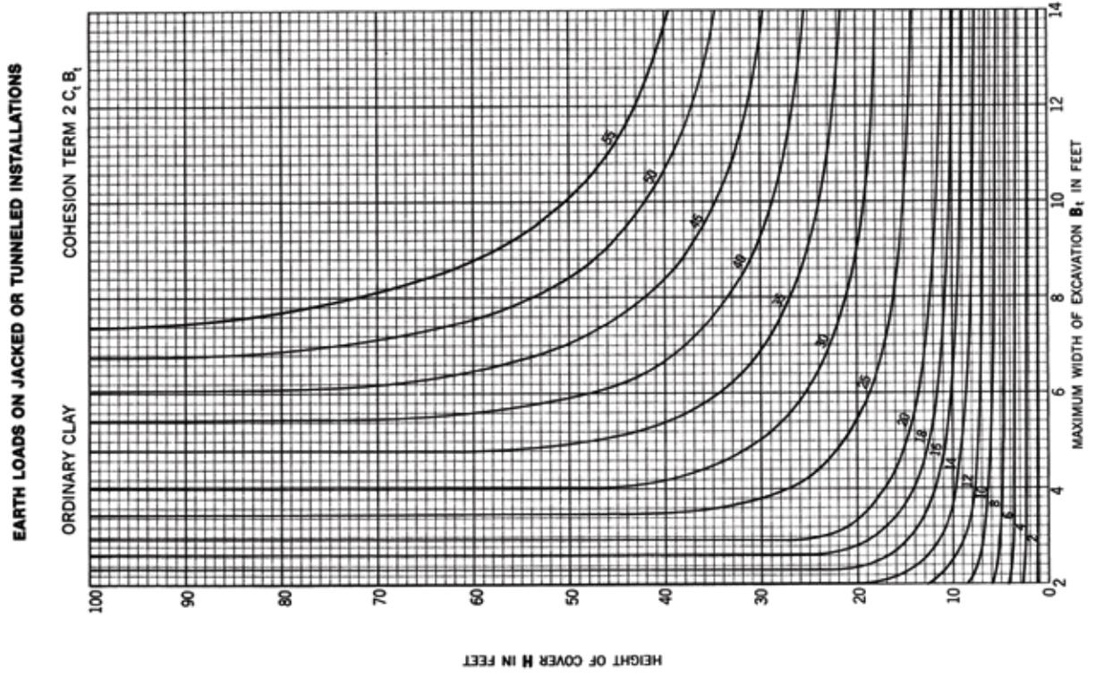
**Figure 8 Earth Loads On Jacked or Tunnelle Installations**
