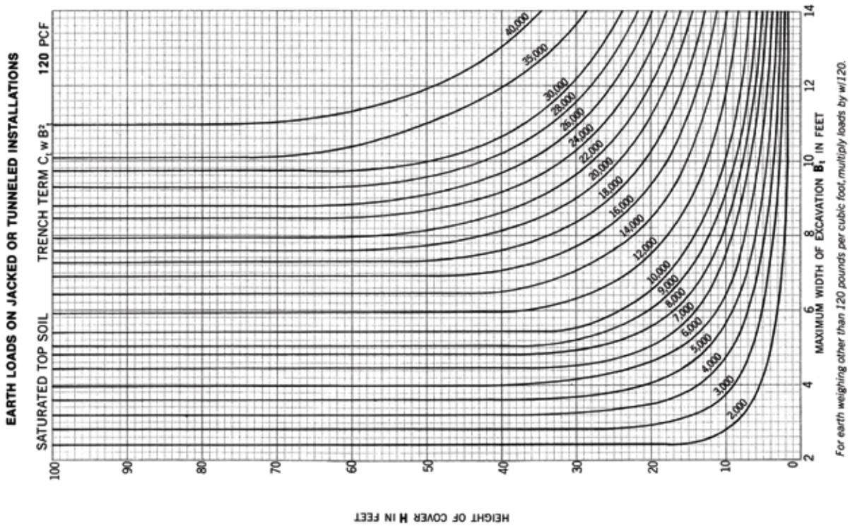
**Figure 5 Earth Loads On Jacked or Tunnelle Installations**
