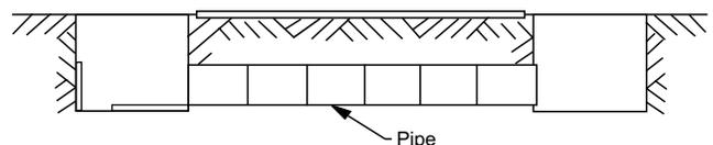
The next section of pipe is lowered into the pit and the above steps repeated. The entire process above is repeated until the operation is complete.
