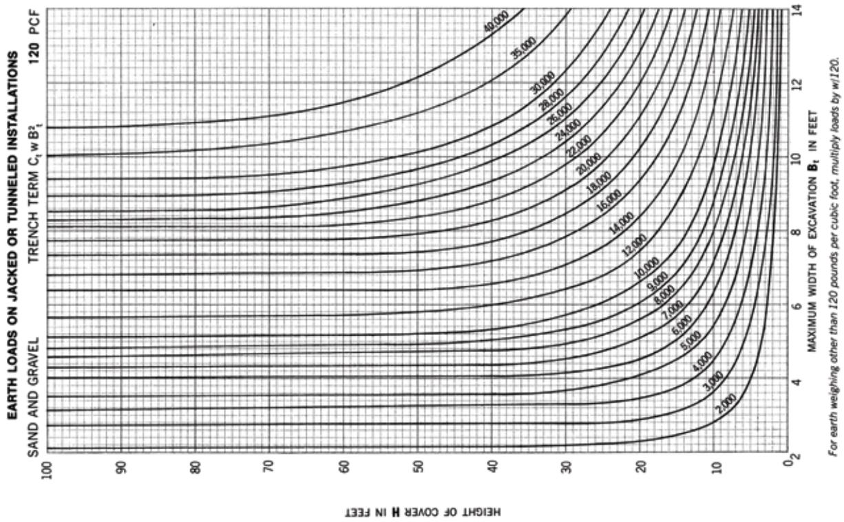
**Figure 4 Earth Loads On Jacked or Tunnelle Installations**
