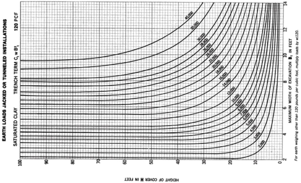
**Figure 9 Earth Loads On Jacked or Tunnelle Installations**
