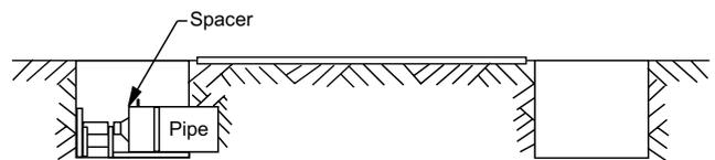
The jack rams are retracted and a "spacer" is added between the jacks and pipe.
