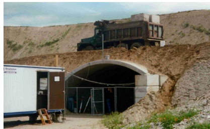
Testing of a BEBO structure, Large Span Culvert Field Test program, University of Massachusetts, 1997.
