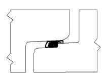
Once fully homed, the compression section seals the total annular space; the rolling tube comes to rest within the small annular space - acting as a cushion against side loads, and the serrations act to resist joint pull-out.
