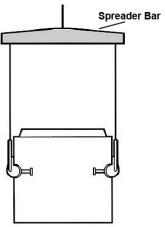
with equal "picking" force on all lifting points.
