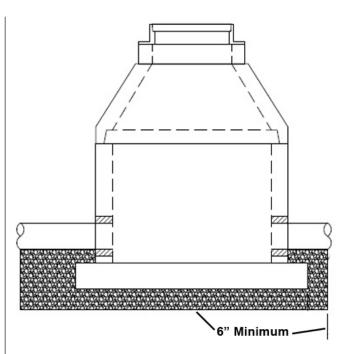
Use a minimum of 6" of approved bedding material compacted to 90% Proctor in an area that is 6" beyond the ouside radius of the manhole base.
